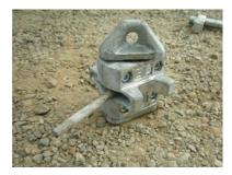
**Double Ended Twist Lock** Double Twist Locks are used to connect two containers together vertically.
